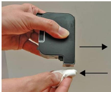
Fig. 0-1: Cleaning the nozzle plate
