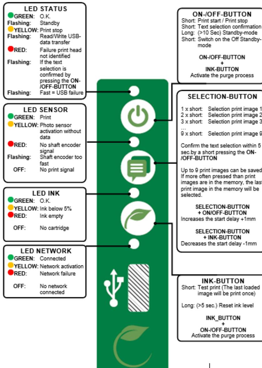
Fig. 0-1: User interface on the top side of the system
