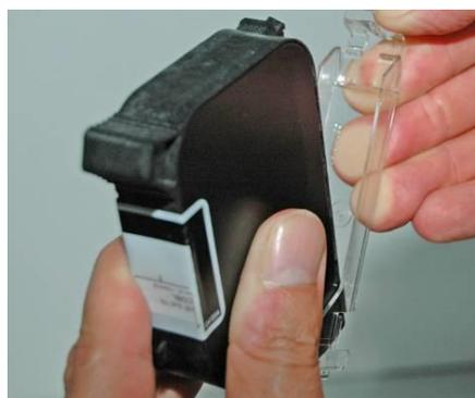
Fig. 4-1: Inserting the HP ink cartridge in the CartClip
