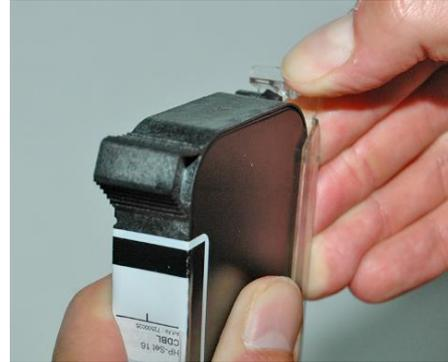
Fig. 4-2: Removing the HP ink cartridge in the CartClip
