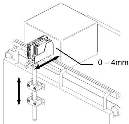
Fig. 0-1: Installation of the Zenjet printer at the production line
