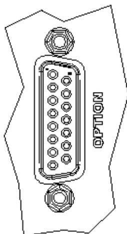
Fig. 0-6: Option-Socket (Sub-D 15-pole) on the system-back and Sensor-LED on the top side of the system
