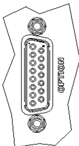
Fig. 0-5: Option-Socket (Sub-D 15-pole) on the system-back and Sensor-LED on the top side of the system
