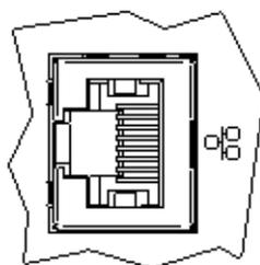
Fig. 0-7: Ethernet-socket (RJ 45) on the system-back and network LED on the top side of the system.
