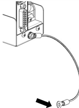
Fig. 0-3: Ground connection at the print system
