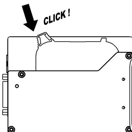
Fig. 0-9: Fixing the ink cartridge
