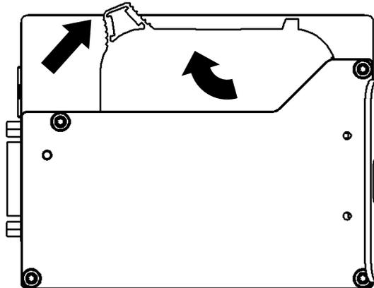
Fig. 0-10: Remove the ink cartridge
