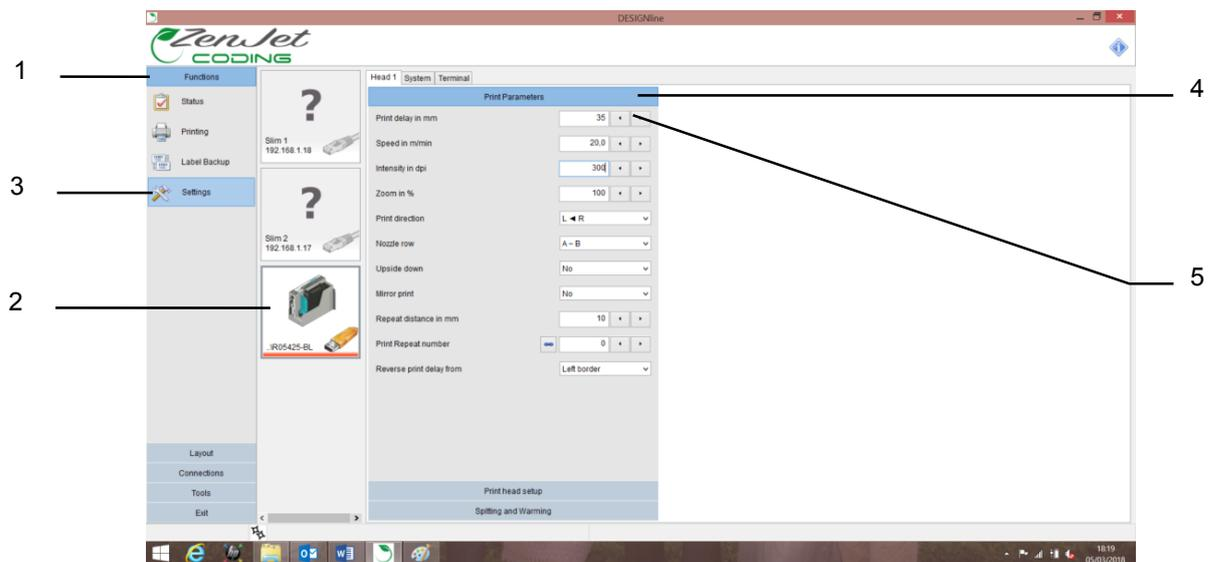
Fig. 0-14: Set up the print start delay in DESIGNline
