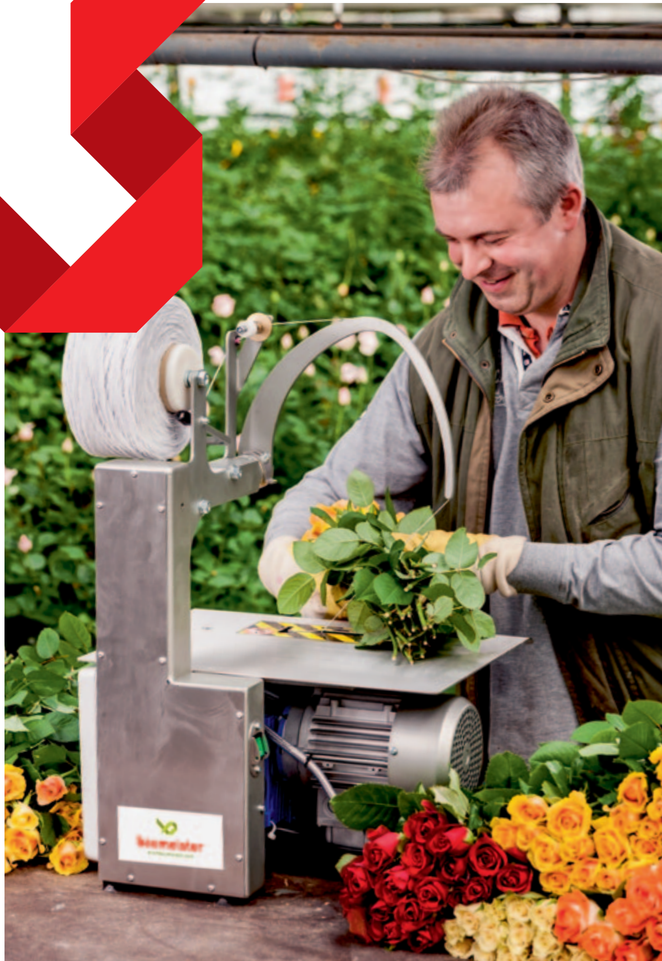
Automatic tying with ADT String-Tying Machine (page 20).
