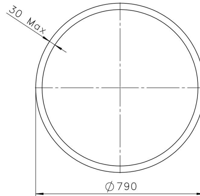
Each item would be stretched from round shape to square/rectangular. This will be possible using 4 pins inside the circle that will move in one axis
