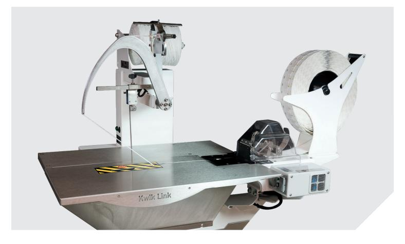
Looking for a way to minimize packaging while providing for branding and traceability? Think Kwik Link! The new Kwik Link is a semiautomatic machine that binds bunches together then adds a closure and label. This results in less packaging for a smaller carbon footprint.
